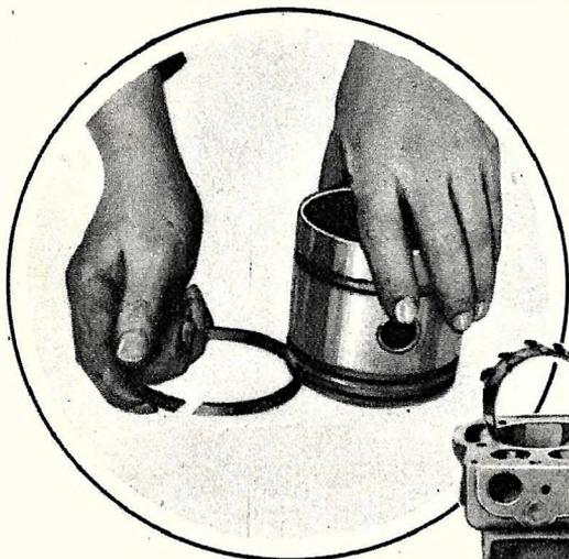
Scrape out carbon deposits from bottom of each piston groove, then fit each ring to its groove by rolling around as shown at left. Mark ring and groove similarly. There should be no up and down motion of ring in groove.
