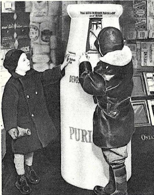
Empty milk bottles deposited in automat reward customer with candy or gum. Sanitary device reduces bottle losses.
