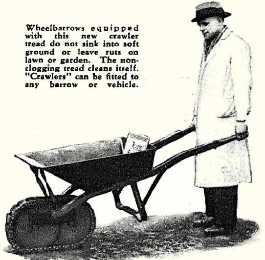
**C**ATERPILLAR treads which can be fitted to garden wheelbarrows are being introduced by a German manufacturer. The new "crawler-barrows" have an advantage over the old single-wheelers since the new vehicle can pass unhindered over soft and sandy soil, thus eliminating the necessity of laying down planks. The barrow is claimed to wheel easily without leaving tracks or ruts on lawns or garden beds.
