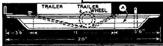
Side view of hull of scow showing how wheels fit into pit.
