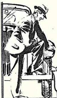
**AIR PRESSURE** in tires should be checked each week. Refill to 2 lbs. over rated pressure, as this amount is normally lost weekly by good tires.
