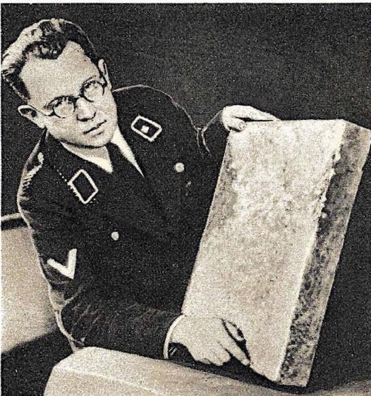
Aretz, famous German chemist, displays a slab of tile made from waste materials. It is a low-cost non-burning insulator.
