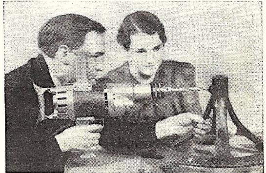
Operating drill made with Ford generator and set of parts.
