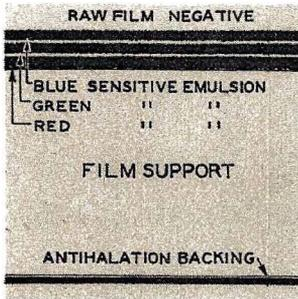
Above sketch shows cross-section of new 16 mm. color film. Note the three-color sensitive emulsions separated by gelatin layers. Ordinary filming requires no filters.
