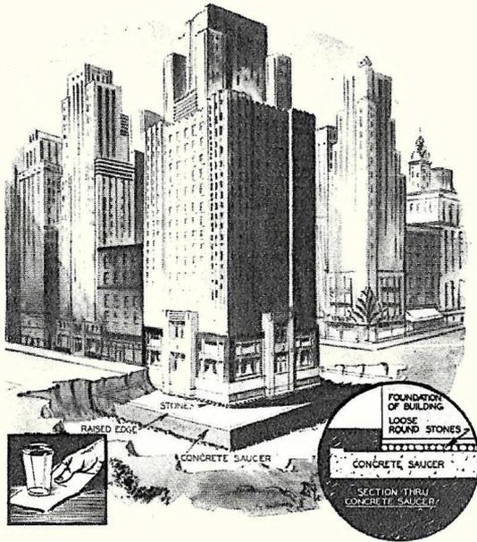
Jerking a sheet of paper suddenly from beneath a tumbler will not upset its contents. On this theory a New Zealand architect has conceived the plan, shown above, for building skyscrapers on a concrete platform covered with round stones to prevent collapse of the tall structures during earthquakes.
