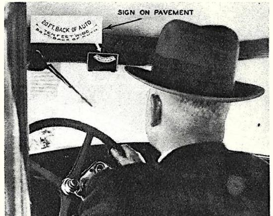
By means of new rear window reflector, image of a sign six by ten feet placed on the road two feet back of the car was reflected into rear view mirror over windshield to show parking advantages of new road-reflecting mirror for motorists.
